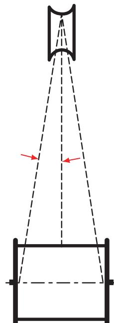
For flat drums it is recommended a fleet angle between 0.5 and 1.5°, and for grooved drums between 0.5 and 2°. If the angle is lower than 0.5° the wire rope will tend to accumulate in any of the drum's surface and if the angle is higher than recommended, there will be friction problems.
